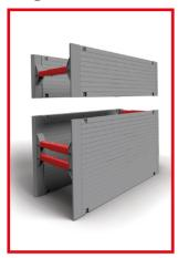
The Drag Box acts as a shield to protect users in self-supporting soil. It is designed to withstand up to 25kN/m². Installation requires the 'Excavate and Drag' technique, the box is placed in a pre-dug trench and moved after each instalment of pipe.
