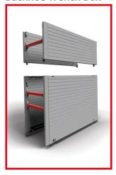
The Backhoe Trench Box is a robust piece of equipment, which acts as a safety shield to provide a safe working area below ground level. For use when working on excavations and pipe laying operations. The Backhoe Trench Box can sustain working earth pressures of up to 20kN/m², users should check that the excavation will not impose greater pressures than this.
