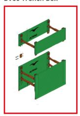
The BV60 Trench box is designed and tested to withstand ground pressure of 23.50 kN/m $^2$ . If ground pressure could exceed this or if the ground is weak or unstable then a temporary works design should be sought from Generation's design department.
