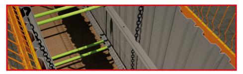
Alloy Waler Rails are used as an alternative to Trench Boxes where cross services are an issue. They are mainly used in city center and highway excavations where ground movement must be kept to a minimum. They offer a two-sided hydraulic support system used in conjunction with Altrad Generation Trench Sheets to allow a clear working area for the inspection/laying of utilities.
