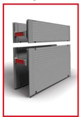
The Maxi Drag Box is ideal for use with long pipe runs, the size increases productivity allowing for a faster installation time. The Maxi Drag Box can be installed using the 'Excavate and Drag' technique. The box is placed in a pre-dug trench and pulled along the trench as each section of pipe laying is completed.
