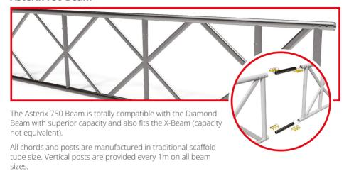
The Asterix 750 Beam also offers consistent node spacing when multiple beams are joined. The node points are spaced to allow connection of a standard scaffold fitting at any point.
