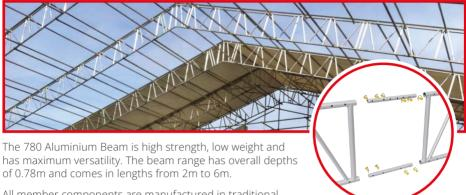
All member components are manufactured in traditional scaffold tube size and vertical posts are provided each 1m on all beam sizes. It also has consistent node spacing when multiple beams are joined, and node points are spaced to connect a standard scaffold fitting at any point.
