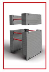
The Backhoe Manhole Box is a four-sided excavation box which provides a safe working area below ground. The Backhoe Manhole Box can sustain earth pressures of 20kN/m². Users should check that the excavation will impose no greater pressures than this.
