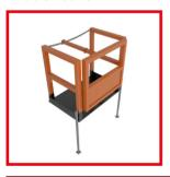
Manufactured from mild steel with a powder coated finish. Specially designed for use on all types of box and sheeted excavations. Cantilevered platform enables safe side-entry onto ladder. Standard pole ladder fits directly onto the unit and is locked in place with two ladder clamps. Adjustable clamps fit directly onto a Trench Box or sheets (two sheet clamps and two box clamps supplied with platform). Adjustable front legs for ease of levelling. Collapsible sides and gate for ease of storage.
