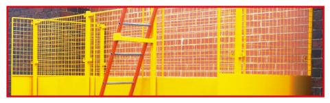
The 3.9m Trestle Handrail System is a simple and easy to erect system used in conjunction with adjustable steel trestles which has been specially developed to meet the needs of the Working at Height Regulations. Using only four components a full hand rail, complete with brick guard, toeboard and stabilisation can be erected in minutes.
